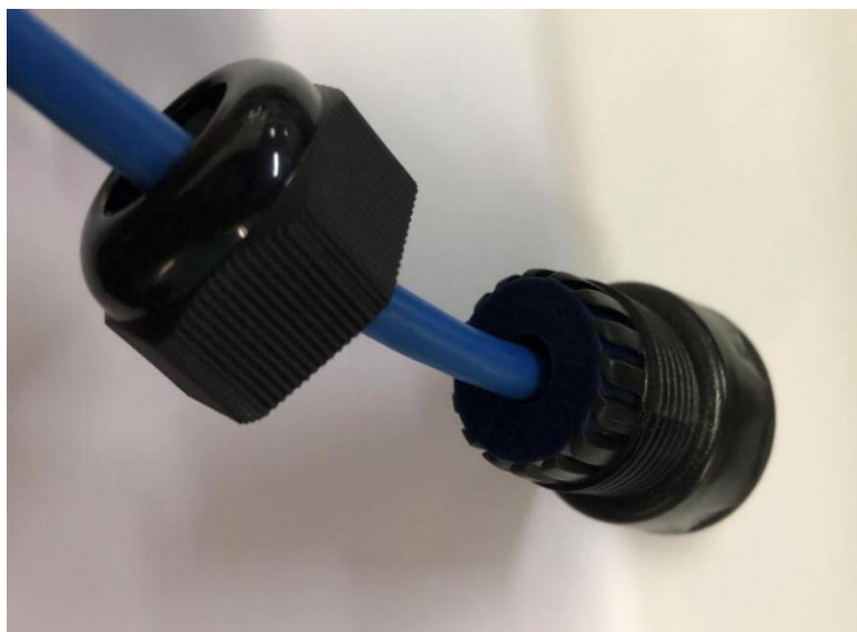
(c) 将密封圈嵌入到卡槽
