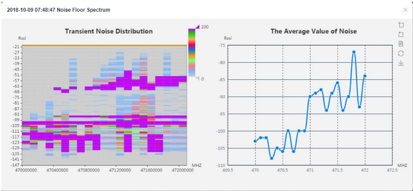
Figure 4-10 Noise canning example @470 to 472MHz
