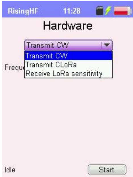
Transmit CW: to transmit unmodulated CW.
