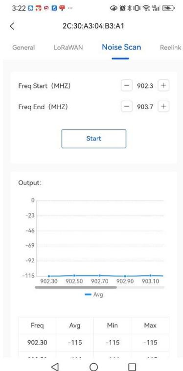
Noise scan mode is used to check the background noise signal level , the scan bandwidth is set to 200KHz.
