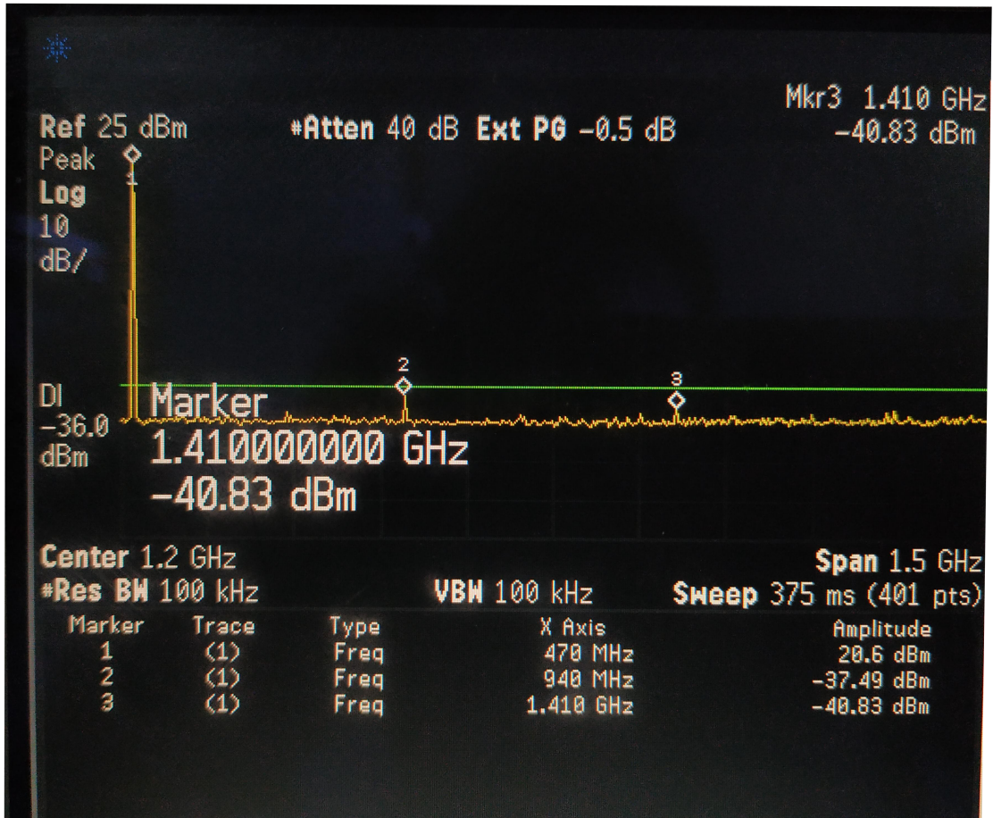
Figure 8 Harmonics measurement @Frf=470MHz, TXOP=21dBm (470MHz)
