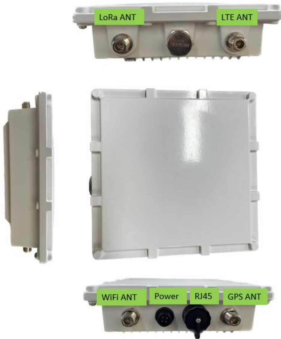
Figure 1 External interface of gateway device
