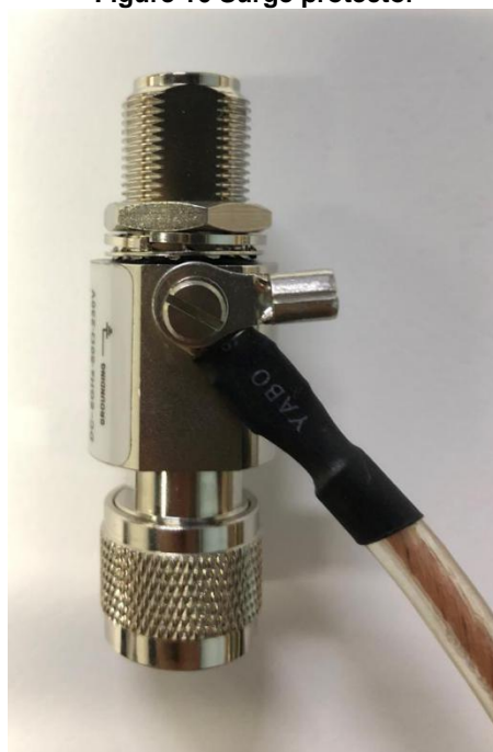
Figure 17 Grounding cable for the Surge protector
