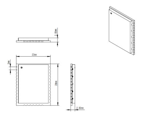
The following figure shows the recommended Layout package size:
