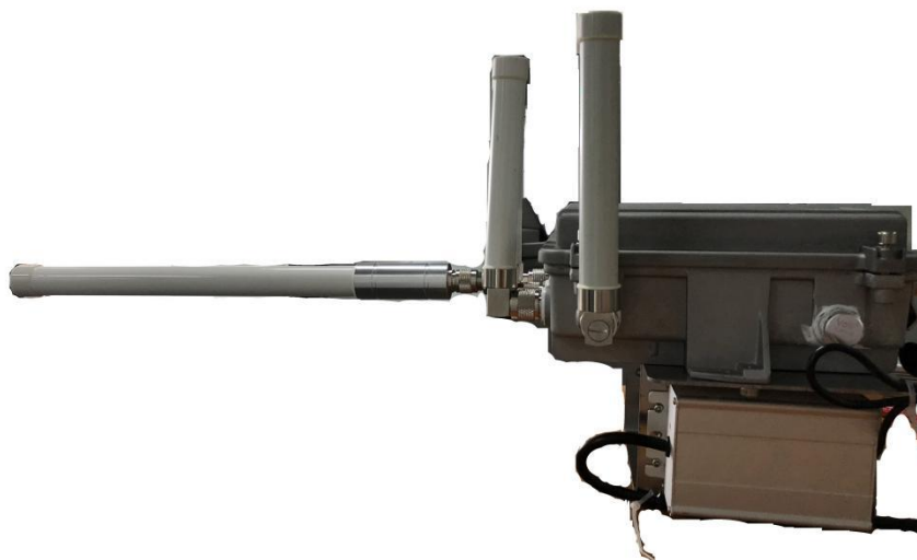
Figure 4-19 Side view of the gateway after installing the antenna
