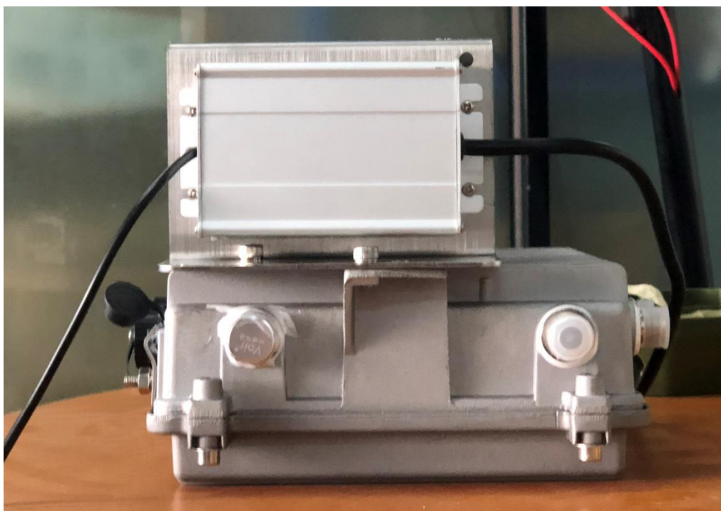
Figure 4-11 Power adapter installation
