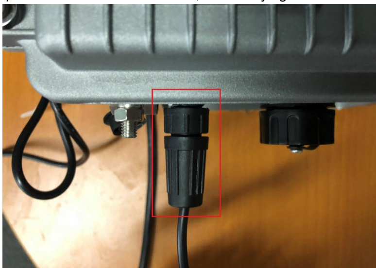
Figure 4-15 Install the power plug
