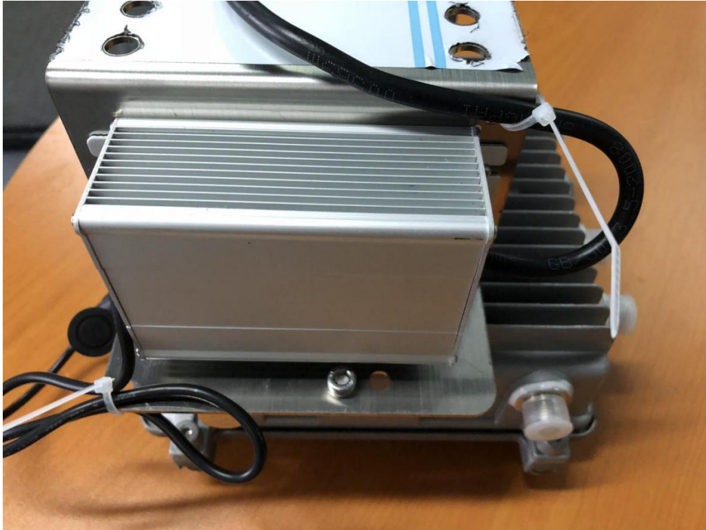
Figure 4-16 Secure the cable with a cable tie
