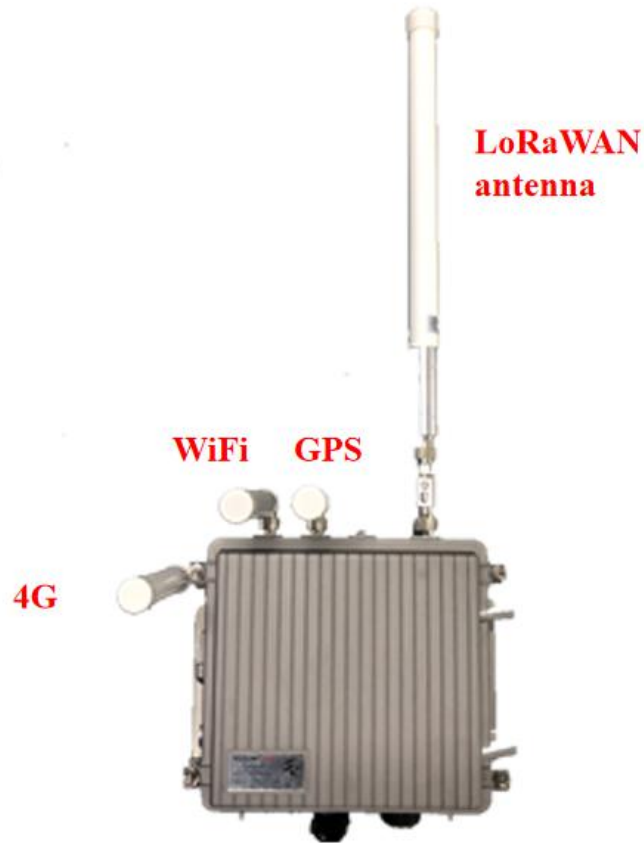
Figure 4-18 Front View of the gateway after installing the antenna
