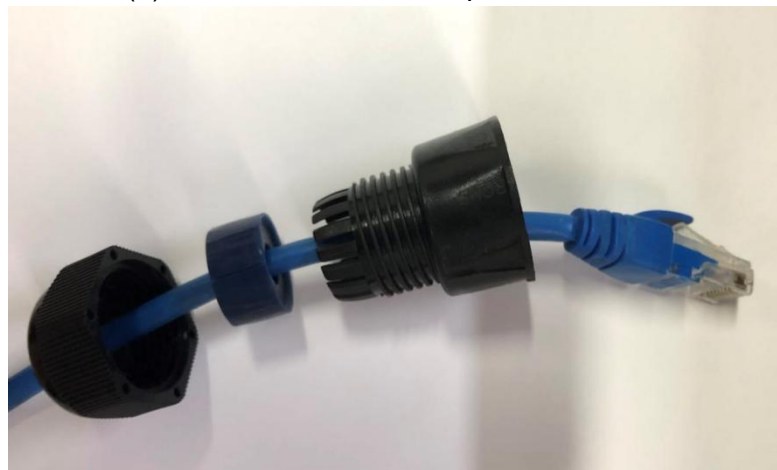
(b) Access the network cable in sequence
